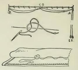
The sketch above shows the arrangement of cord and pulleys for draw curtains. The method of lining a curtain is shown below.
